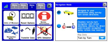
Select the Navigation Mode button in Menu 3 to access the Navigation Mode screen. The Navigation Mode screen allows you to switch between the unit's two different navigation modes.
